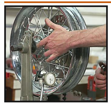
If your motorcycle has spoke wheels, spoke inspection and maintenance is very important. Loose spokes will not only adversely affect handling, but will also damage your wheel hub. If not maintained, lateral and radial rim run out will change and a wobble will occur.
