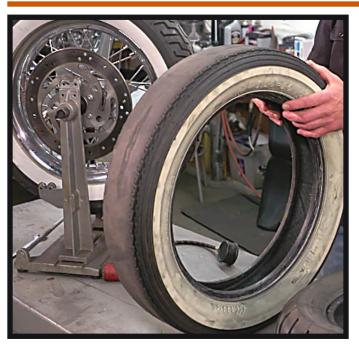
The tire pressure and tire condition are probably the most overlooked area of a motorcycle. Running bald or damaged tires on a motorcycle is extremely dangerous. Check your tire pressure at least once a month. Better yet, check before every ride. When buying new tires, look for the date they were made. Put a hand on them and feel for any cupping.
