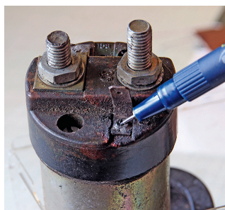
Carefully unsolder the connection to get inside the starter solenoid.
