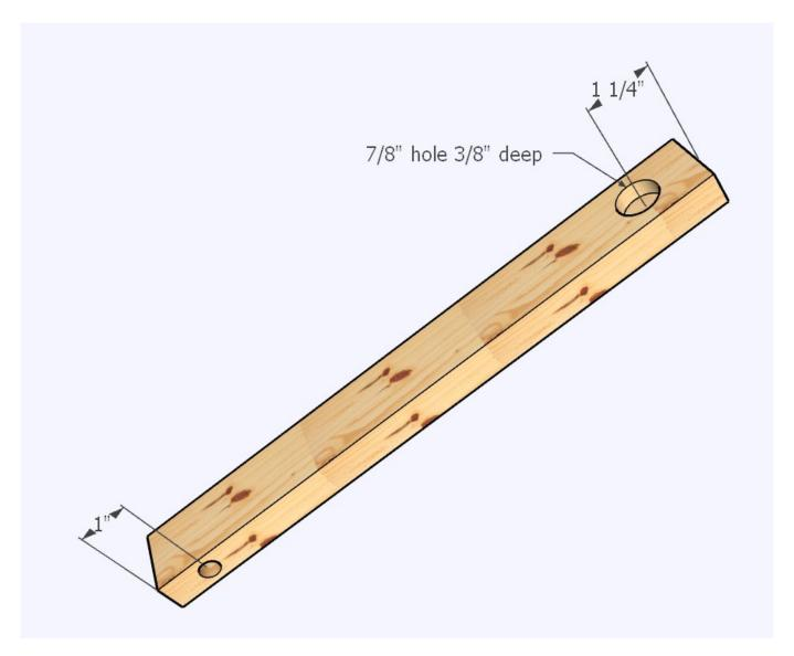
The arm requires two holes. The dowel hole is 7/16" diameter and goes all the way through. The marshmallow cup is counterbored 3/8" deep.
