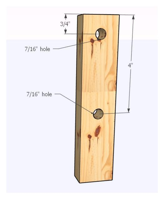
The uprights get two holes, both are 7/16" diameter. The holes are centered on the width of the uprights and the dimensions given to locate the holes relative to the end are to the center of each hole.
