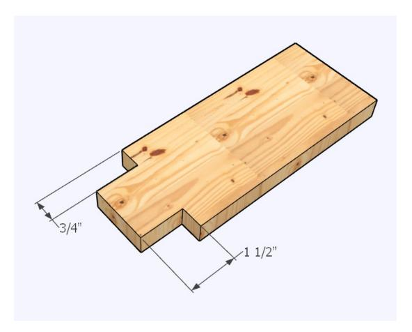
Cut notches or shoulders in the base for the uprights to fit into. When you assemble the catapult use glue, brads and, if necessary, screws, to secure the uprights to the base.
