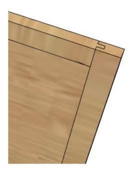
Use a tongue and groove bit set (See Sources) to create the door joint.
