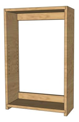
Construction of the cabinet case is very standard with the top captured in a rabbet and the bottom or deck captured in a dado. Two screw cleats in the back of the cabinet provide the rigidity you need to hang the cabinet on a wall. The case sides also include adjustable shelf holes. These are commonly 1/4" or 5 mm diameter to match readily available shelf pins. Center the banks of holes vertically, per the video.
