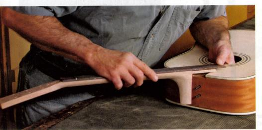
A crucial joint simplified, but only a little. In many kits, the neck attaches to the body with a couple of bolts instead of a dovetailed key. The dovetailed key is more traditional, but many makers use a bolt-on neck for ease of construction and repair. You may need to carefully sand the neck's heel to adjust the fit and ensure that the neck meets the body at the correct angle.
