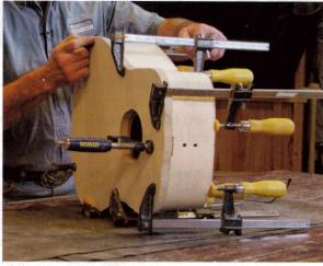
How to avoid specialty clamps. Gluing up the sound box typically requires 25 to 30 luthier's spool clamps for even pressure around the top. Vondriska uses a few ordinary bar clamps and a guitar-shaped caul to distribute pressure.
