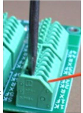
**Connect sensor pair 1:** Connect the orange (or red) wire from the IR LED to terminal 1K. Connect the green (or blue) wire from the IR receiver to terminal 1F. How you connect the two white (or yellow) wires to the MRD6X will determine whether Detector 1 will operate in 'Across the Track' or 'Reflective' mode. See the diagrams below.
