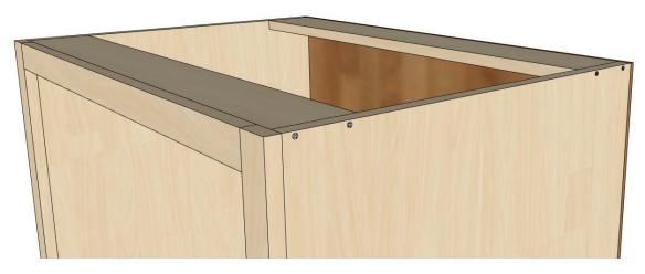
Assembly is very simple. The case is put together with butt joints, glue and screws. Pocket holes hold the face frame together. Use two pocket holes on each end of each face frame rail.
