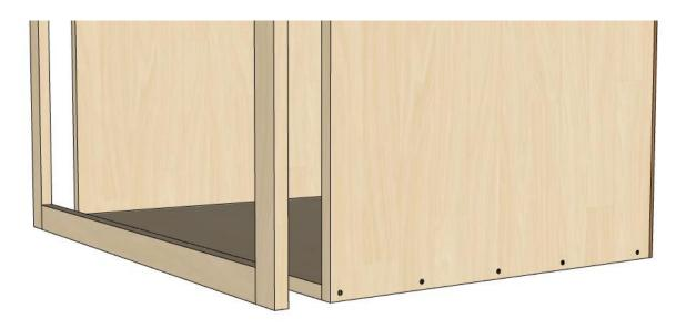
The case bottom is flush with the bottom edge of the case side. The top edge of the lower face frame rail is above the top face of the case bottom, which helps prevent your vac from rolling out of the cabinet.
