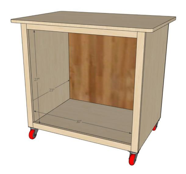
Double check the project dimensions to make sure your vac will fit in the cabinet alongside your Dustopper. Adjust the dimensions as needed.
