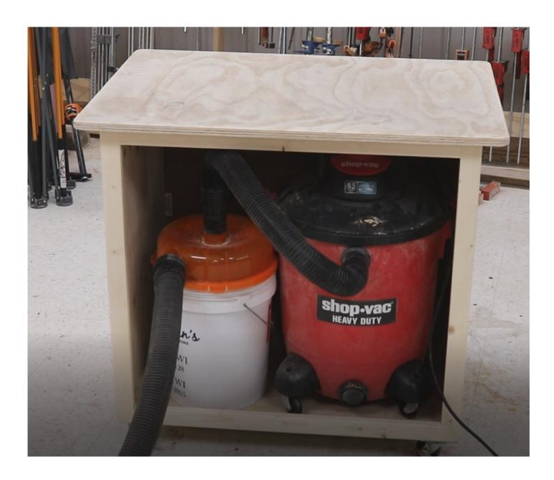
This easy-to-build cabinet will house your shop vacuum AND Dustopper. It provides a work surface you can use portable power tools on (while keeping them hooked up to your vac), and you can roll it around your shop for general clean up. And, the case can be made from one sheet of 3/4" plywood.
